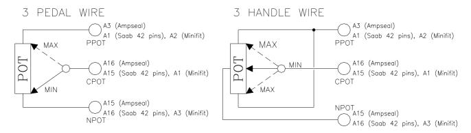
The Procedure for automatic potentiometer signal acquisition is carried out using the Console. This enables adjustment of the minimum and maximum useful signal level (PROGRAM VACC function, see Chapter 9.4), in either direction. This function is unique when it is necessary to compensate for asymmetry with the mechanical elements associated with the potentiometer, especially relating to the minimum level. The sequence of procedure is described in the programming console manual.
