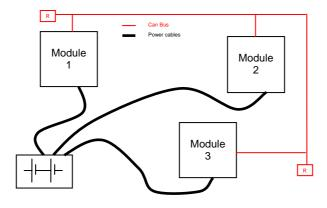
The red lines are can wires.
