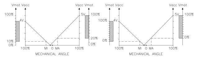
The two graphs show the output voltage from a non-calibrated potentiometer with respect to the mechanical "zero" of the control lever. MI and MA indicate the point where the direction switches close. 0 represents the mechanical zero of the rotation.
