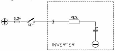
If the charging procedure is incorrect, an alarm is signalled and the main contactor is not closed.
