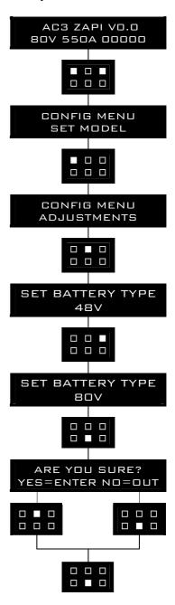
Flow chart showing how to carry out ADJUSTMENT BATTERY operation by console.
